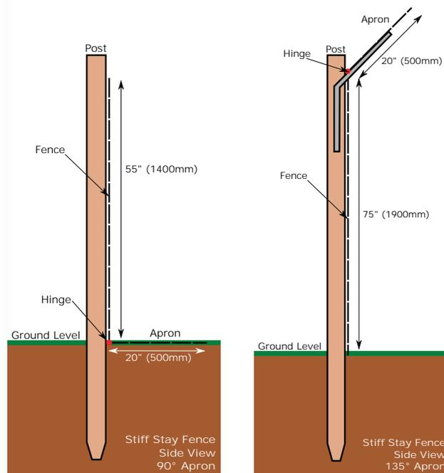
Both the height of the fence and the length of the apron can be configured to suit individual needs. The apron can be placed at any angle depending on the application.
